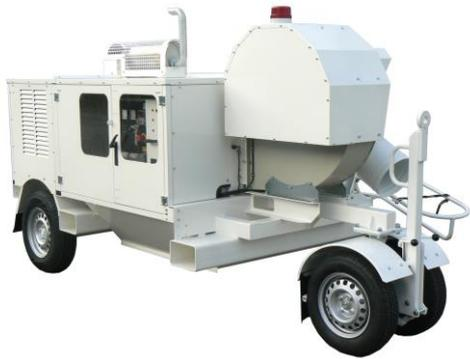
Polar GSH-W20 is a heavy-duty ground heater for wide body aircraft. Utilizing a large blower, electrically powered by a Deutz 4-cylinder diesel and a generator, the unit moves the heating air efficiently throughout the whole fuselage of the aircraft.
